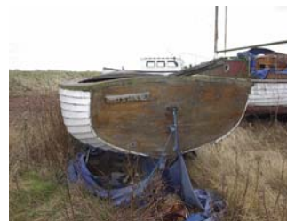
LISA LAN is a Mapleleaf and built at this yard where she now languishes. She is in a poor state with two top strakes rotten and the cabin sides completely missing by the doghouse. She still has most of the interior and engine intact which shows inside that she could be a very comfortable yacht
