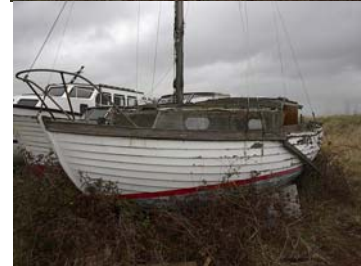
LISA LAN is a Mapleleaf and built at this yard where she now languishes. She is in a poor state with two top strakes rotten and the cabin sides completely missing by the doghouse. She still has most of the interior and engine intact which shows inside that she could be a very comfortable yacht
