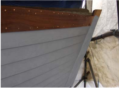
First coat of primer on starboard side
