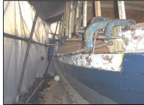
The forward scarf was particularly awkward to squeeze the planks in line due to the curve in the hull.
