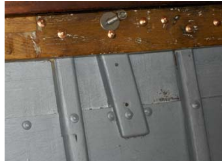
Oak backing for shroud plate fastened to planks
