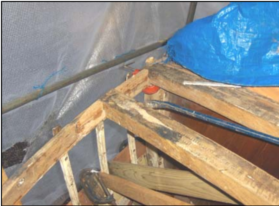
The Carling had to be replaced in two sections, but as the original had casellations that extended through half of the wood in any case I deemed that this would not be an issue. I also had to take care to try and keep the shape of the boat as a lot had been removed, hence the braces.
