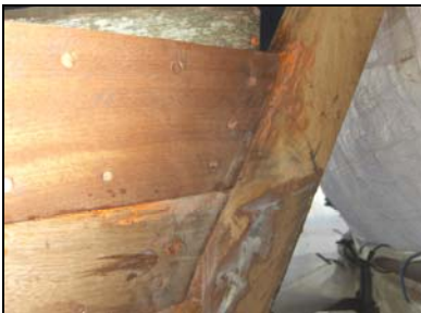
Fastening the bow end of the plank
