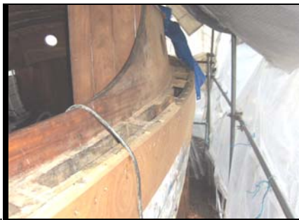
Void between carling and top plank filled with oak and riveted through
