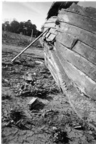
Fig 1. CATHY's hogged keel. She had just one sleeper positioned under the centre plate pivot.
